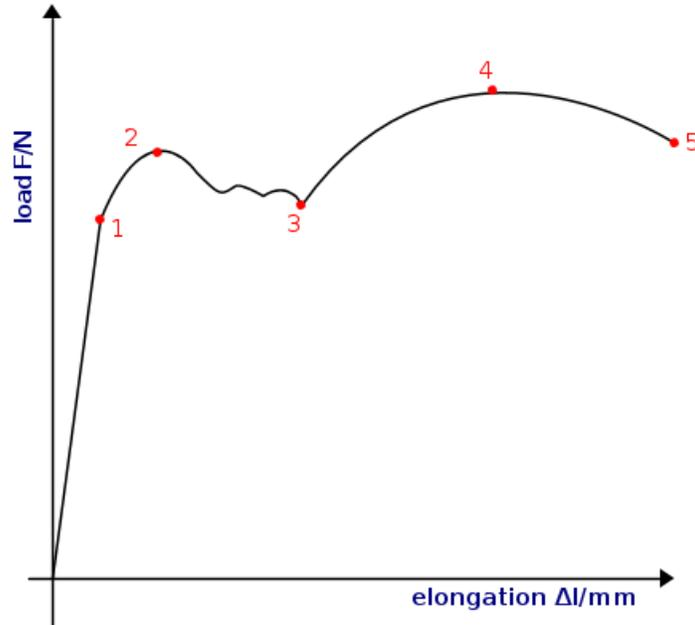
From the stress-strain curve it is possible to extract some characteristic values, that are:
