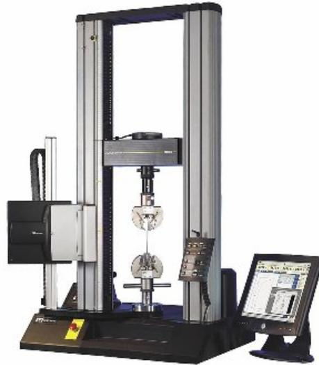
The load must be increased from zero up to the end of the test, so that its increase is constant. Before the test, the machine must be calibrated. Moreover the gripping of specimen's shoulders must be such as to obtain a distribution of a uniaxial tension in the same specimen.
